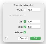
Enable *Width* to assign a new width to all selected glyphs. Check *on both sides* to modify both sides equally to match the new width. Otherwise, the points on the layer keep their original coordinates.
