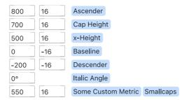
The left number field of a metric defines the offset from the baseline. (The *Italic Angle* metric has one field only.) The right number field is the size of the alignment zone and starts at the offset of the metric. Nodes and anchors placed in alignment zones are highlighted. See section 4.2.5, 'Nodes in Alignment Zones' (p. 25) and section 4.4.1, 'Adding, Editing, and Removing Anchors' (p. 35).
